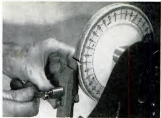
PROTRACTOR EDGES are concentric with a center hole. Simple pointer is cut from a sheet of aluminum
